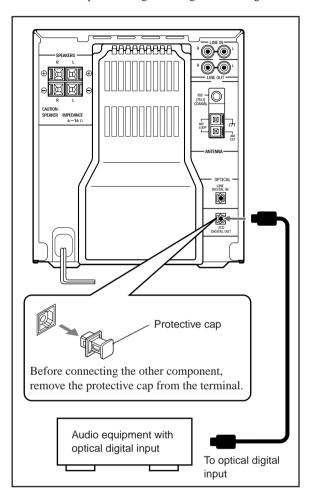
Connect between the optical digital input terminal on the other component and the 3CD DIGITAL OUT terminal.
